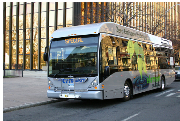
Fig. 5. Hybrid-electric fuel cell transit bus operated by CT Transit, Hartford, CT.
