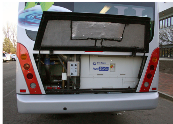
Fig. 4. PureMotion® Model 120 fuel cell power module installed in a transit bus engine bay.
